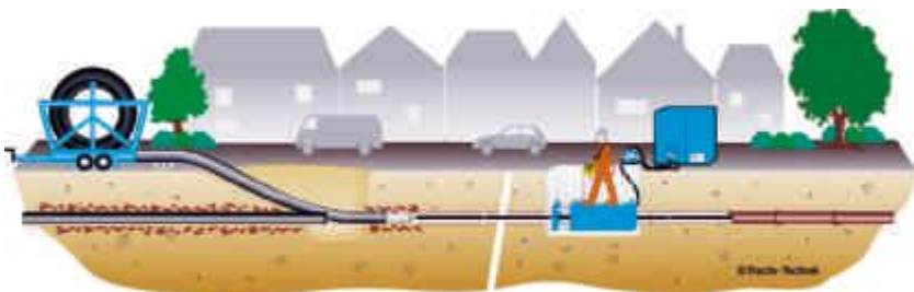
Fig. 1.1: Layout of a modern pipe bursting process
